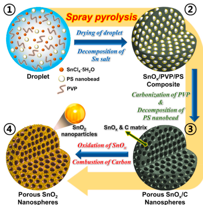
Scheme 1. Schematic illustrates the formation mechanism of porous SnO 2 nanospheres using one-step spray pyrolysis process.
